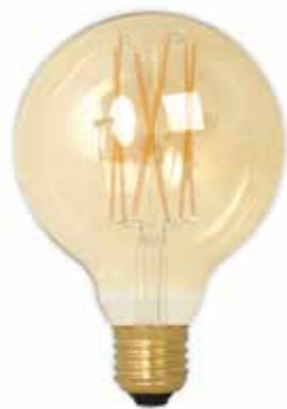
3. LED Filament Globe Gold Finish CAL-425464. ES, G95 (Globe) 95 x 140mm. Efficiency A+; 4W; 320 Lumens; 2100 Kelvin; Dimmable
