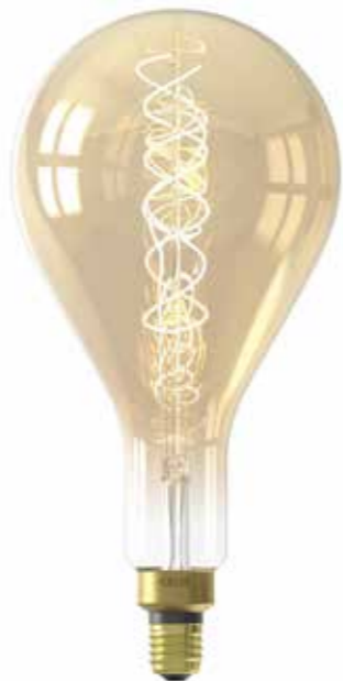
2. LED Full Glass Flex Filament Splash CAL-425812. ES, (Globe) 161 x 330mm. Efficiency A; 4W; 200 Lumens; 2100 Kelvin; Dimmable
